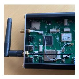
12. To connect the connection board for the dual version to the Larus board, you need an approximately 8cm long, 6-wire cable that has a JST GH 1.25mm connector on one side and a Molex connector 51021-0600 on the other side has.
