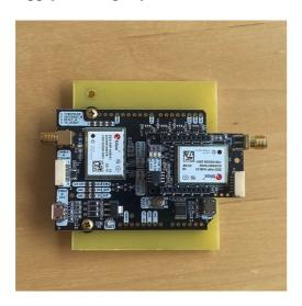
21. Shorten the screw under the small circuit board flush with the nut, otherwise it will not fit over the standing USB-C socket later.
