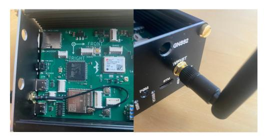
11. Installs the cable for the GPS antenna in the Essential.
